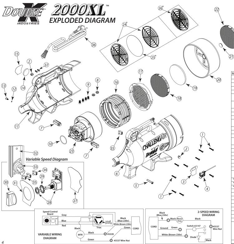
\* Part #s 2177, 2178, and 2100 have been replaced with part #2191. Dryers produced after January 2011 will have #2191 internal filter housing with filter #2196 installed.
